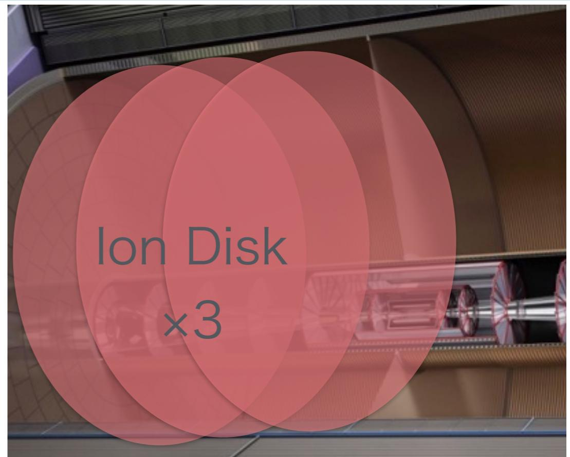
The ions for a single bunch train form a disk with about 1cm thickness.
