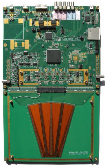
Fig. 6: Photograph of a LumiCal readout module attached to a sensor.
