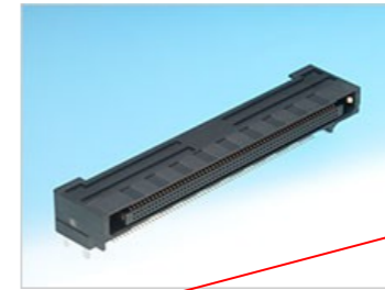
Core Module connector: 7 common differential pairs for sensitive signals, 30 individual pairs for control and readout, 14 common lines, GND
