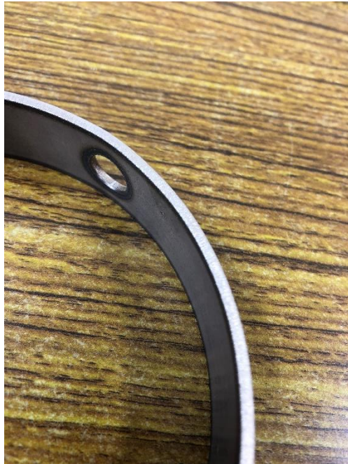
Stiffener rings cut by a laser beam
