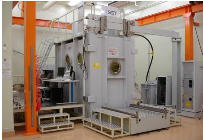
EB welding machine (SST, Germany) Max. beam voltage: 150 kv
