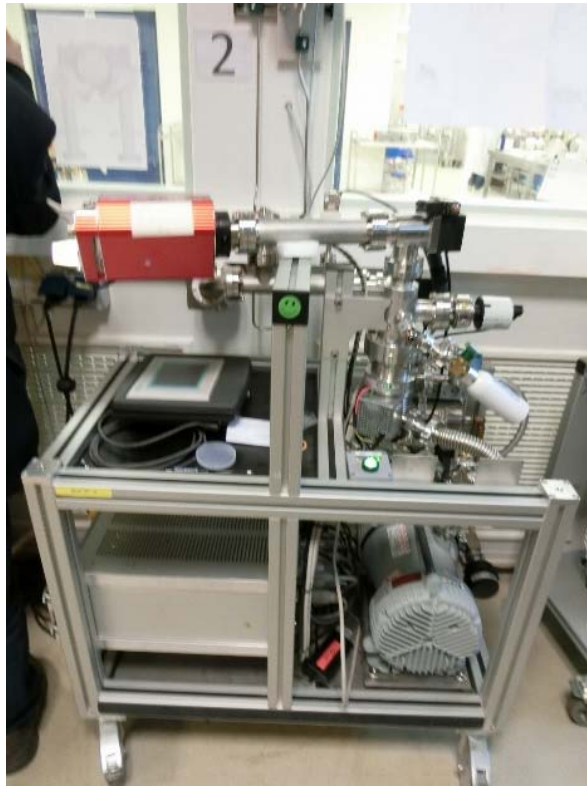
slow pumping & venting system (Euro-XFEL)
