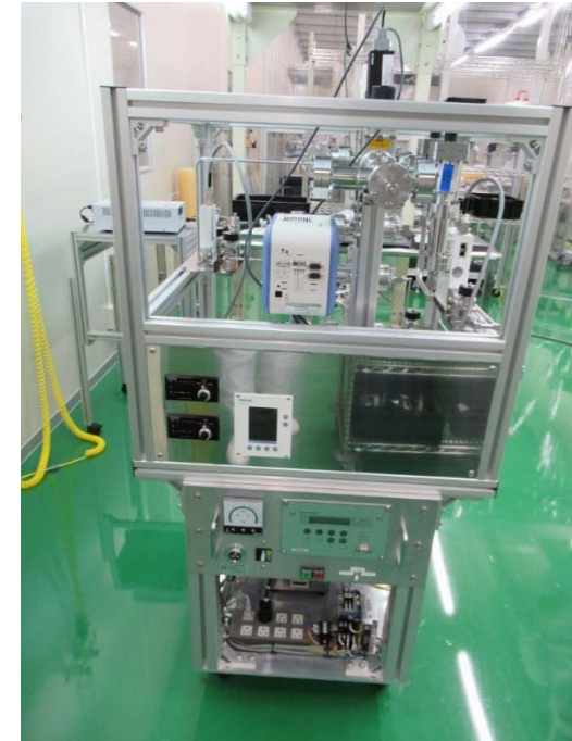
Slow pumping & venting system (in KEK)
