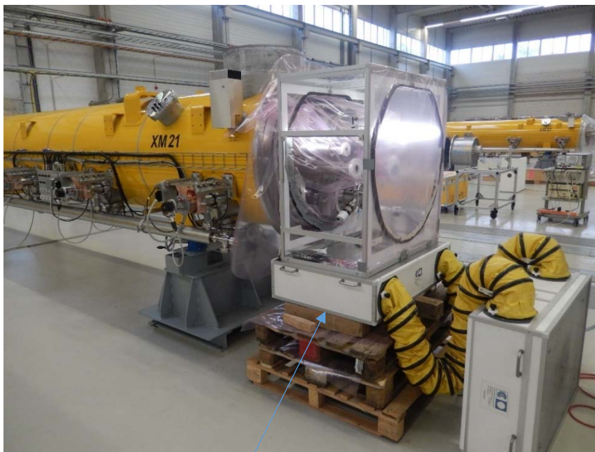
local clean booth with laminar flow (E-XFEL)
