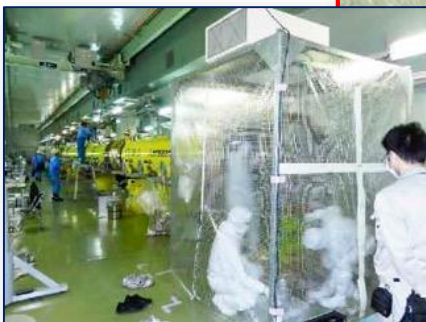
Local clean-room with down flow clean air
