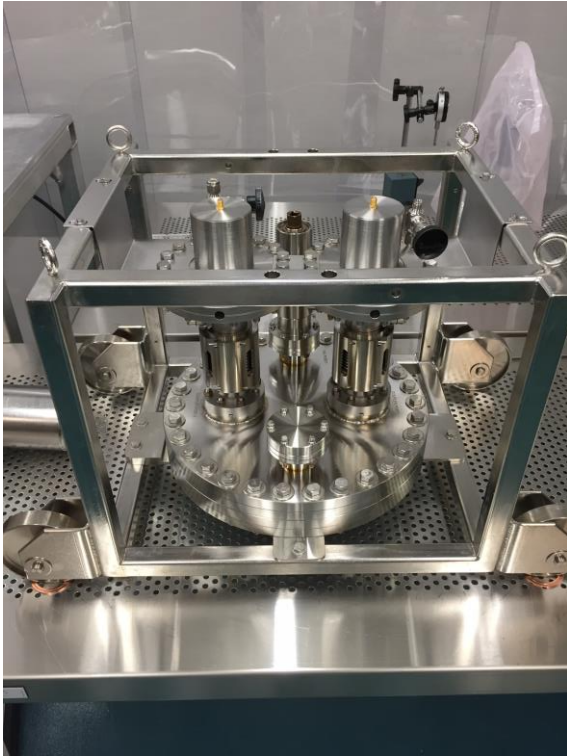
Pair of cold assemblies as received on test stand
