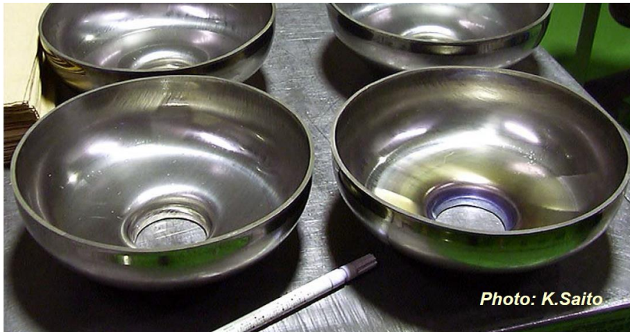
JLab-style LL cavity-shaped half cells x 4 (Nb, 4mm-t)
