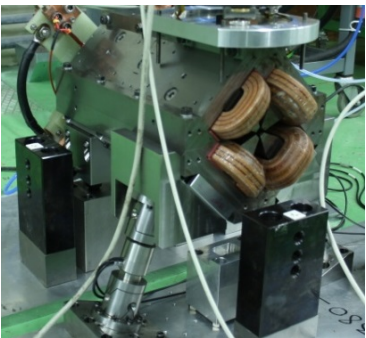
Main Beam Quadrupole
