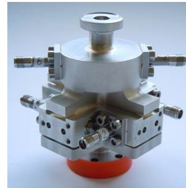
Beam Position Monitor (BPM)
