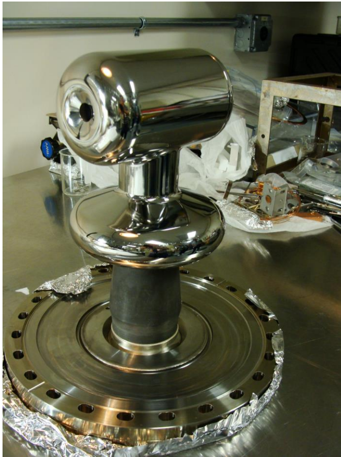
CEBAF 200 kV Installed June 2018 (operates at 130kV until an upgrade in 2020)
