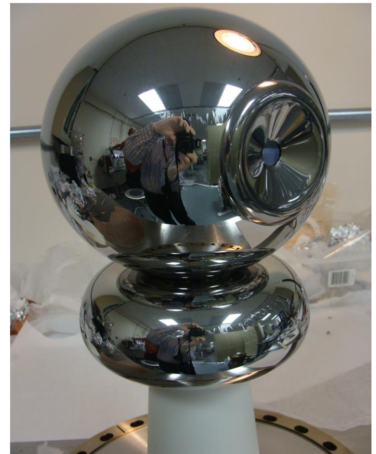
UITF 350 kV Polarized Gun Under assembly
