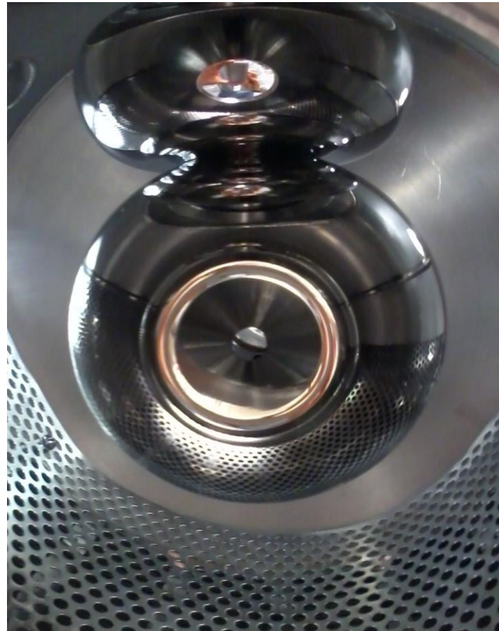
GTS 350 kV In operation since Nov 2016 with CsK 2 Sb photocathode
