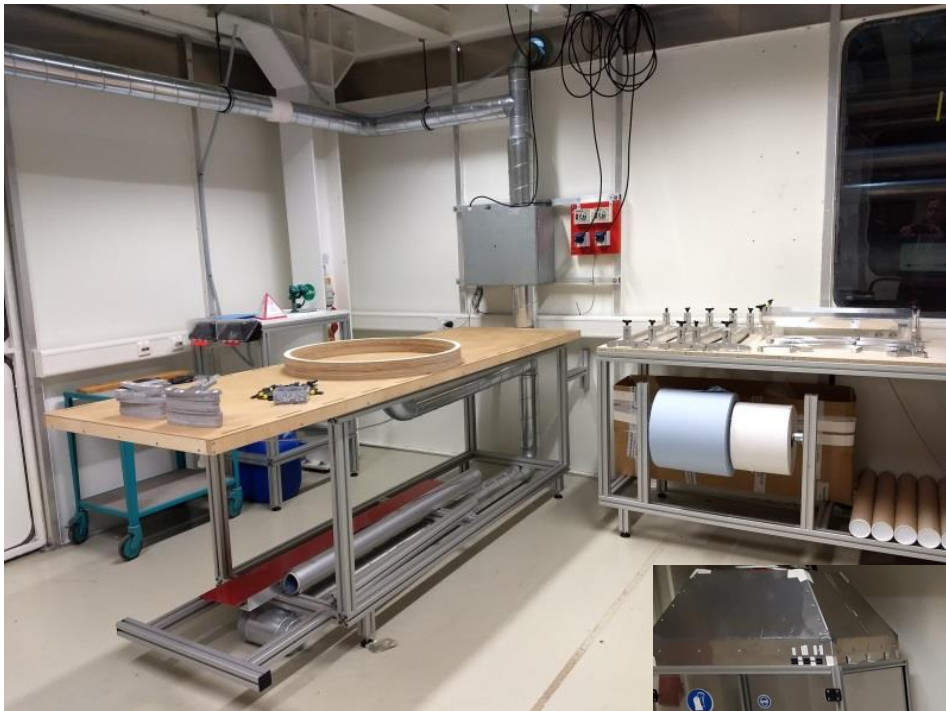
„Gluing“ room, preparation table incl. end flanges of the new field cage (Bernd Beyer)
