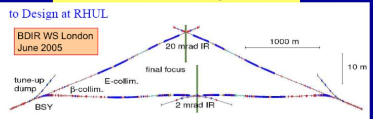
Full optics for all beamlines, 2 mRad and 20 mRad designs explored in detail, up/downstream instrumentation present for both IRs.
