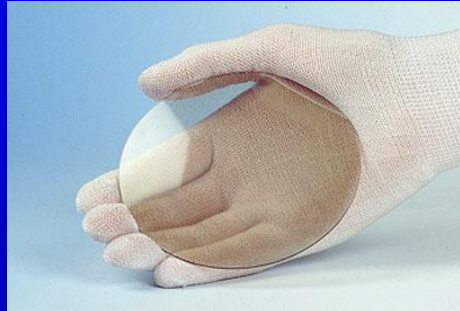
polycrystalline CVD diamond wafer (Photo: IAF)
