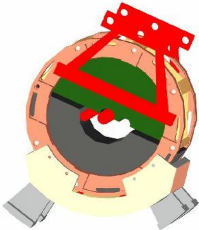
**Fig 5. BeamCal installation scheme. Phase 2:** *Parts are fixed together and rotated clockwise.*
