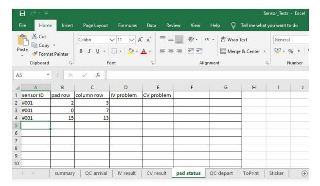
Pad status: sensor ID associated with the (x, y) problems with IV or CV measurements.
