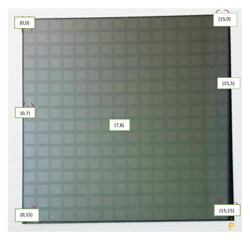
Here a photo illustrating the location of each pad on the sensor.
