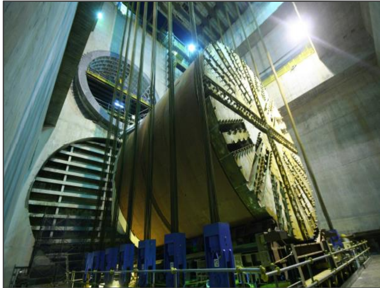
Shield Machine: Gross weight 2100 tf
