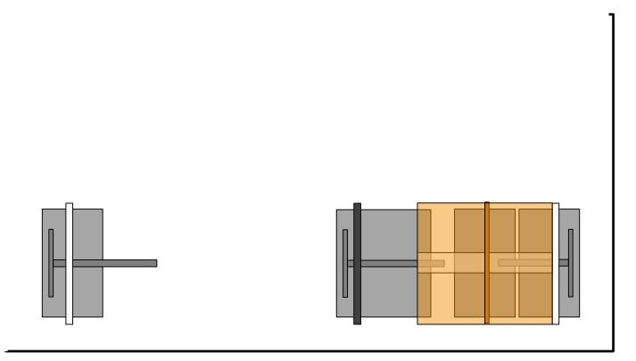
Alternative: First fixing of inner vessel in field cage, then installation / spanning of cathode.
