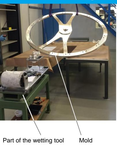
Wetting tool and mold for an T-Shape cross section rim from NIKHEF, designed for the Atlas Endcap 2m outer dia
