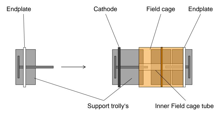
Alternative: First fixing of inner vessel in field cage, then installation / spanning of cathode. Top view of TPC assembly
