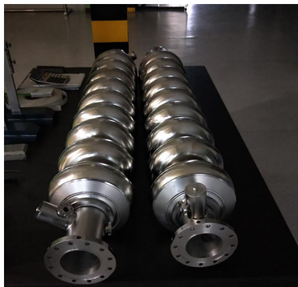
Large grain Nb disc and cavity manufacture
