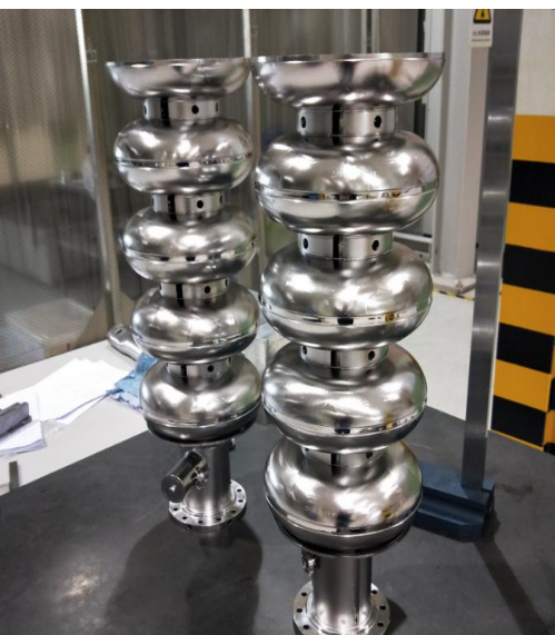
Large grain Nb disc and cavity manufacture
