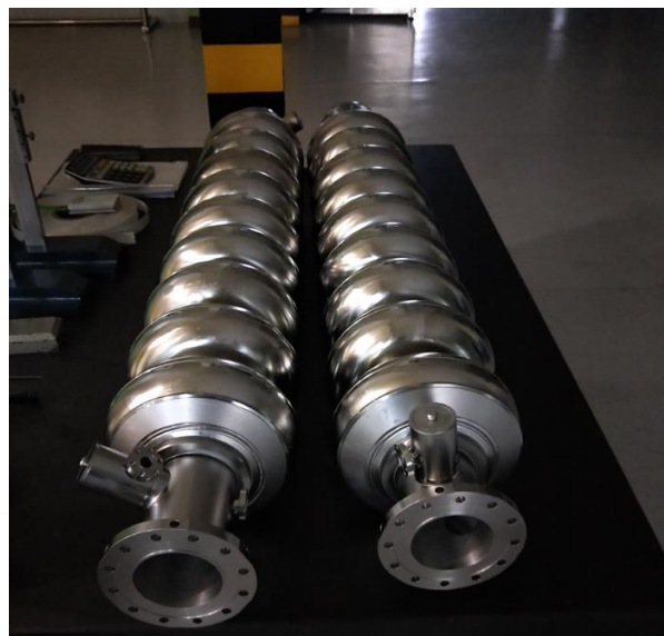
Large grain Nb disc and cavity manufacture
