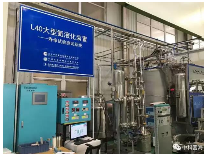
Successful application of 40L/h LHe liquefier (2016)
