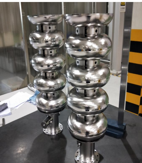
Large grain Nb disc and cavity manufacture
