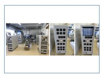
Rack photo with installed modules. Amplifier system can operate after relocating modules. (cold-swap)
