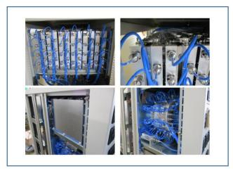
12 pcs of RF "4-Parallel" modules (50kW) and 6 pcs of heatsinks are inserted into the rack.
