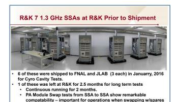
$1300MHz \ge 3.8kW CW-SSA$ 1st Shipment for SSSC Architecture System
