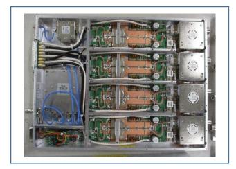
RF "4-Parallel" Module (4.4kW) Inner Photo. 4 solid-state amplifier pallets are equipped in parallel within the module.
