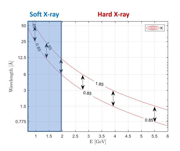
Both undulator lines have identical parameters, so K is tuneable to provide a factor of 2 wavelength tuning for both Soft X-ray and Hard X-ray
