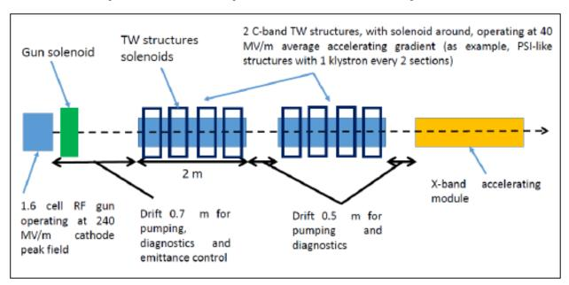
Schematic layout of the C-band injector
