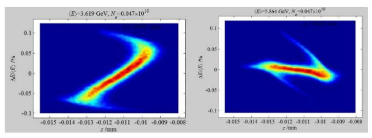
Longitudinal phase space from 1-D tracking at the exit of the linac for SXR FEL (left) and at the exit of the linac for HXR FEL (right)
