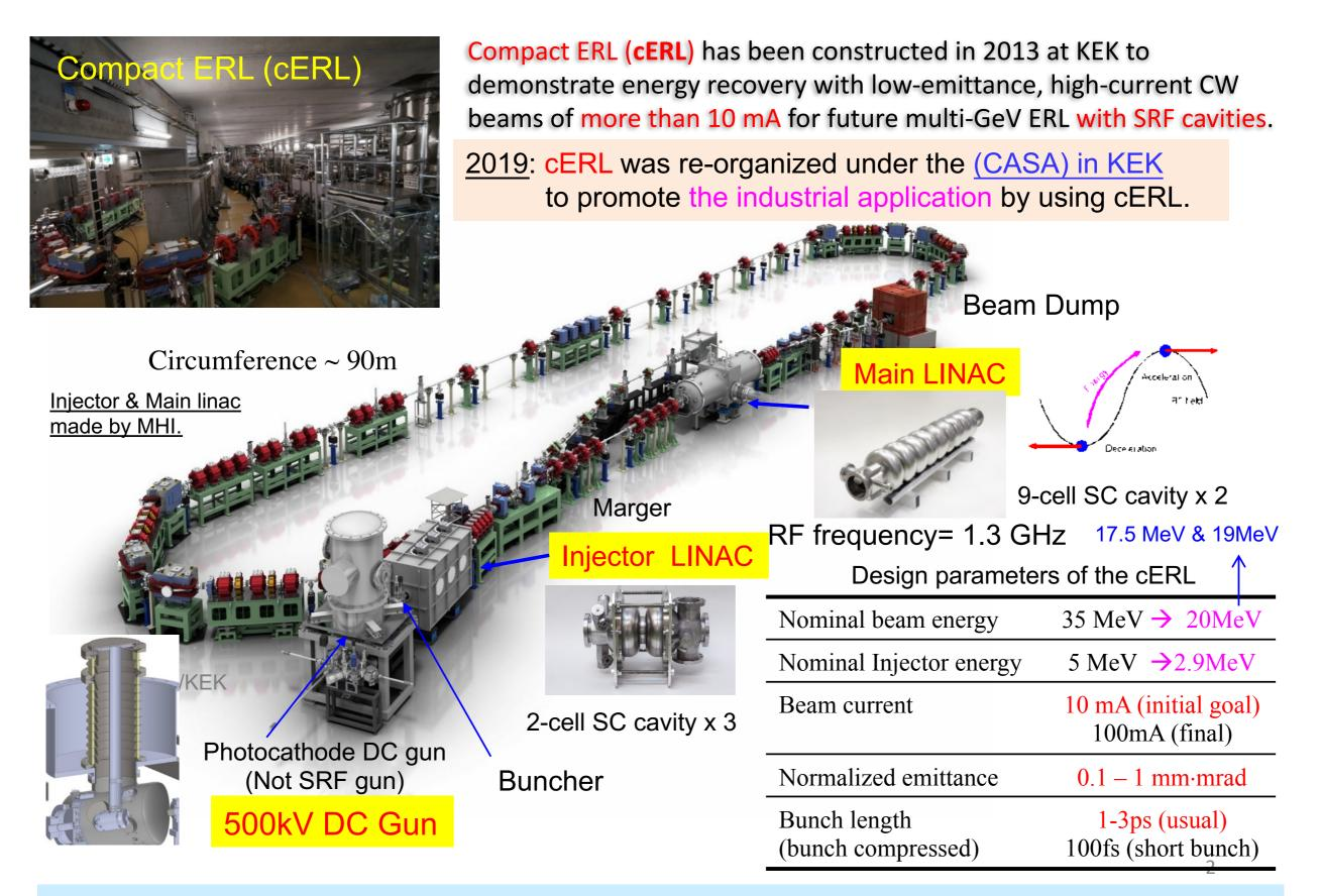
DC gun & SRF linac are based on linear collider technologies  $\rightarrow$  <u>cERL is a real LC application</u>.
