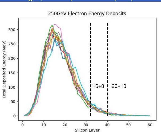
Energy deposition vs layer number in 60 layer simple stack.
