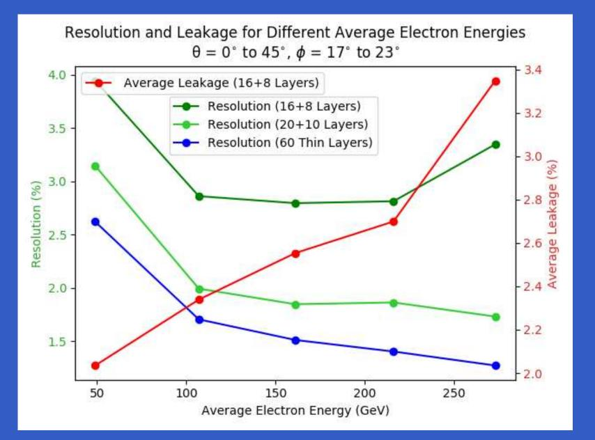
Full ILCsoft simulation. Can the reduced (16+8) ECal performance approach the nominal (20+10) performance with a neural network trained on the 60 layer ECal? LCWS19 October 2019 – p.6/18
