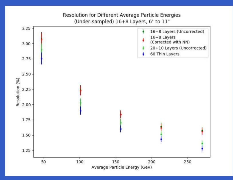
No improvement in resolution due to layer geometry in overlap regions, as expected, since the resolution as already good since leakage is minimal. LCWS19 October 2019 – p.16/18
