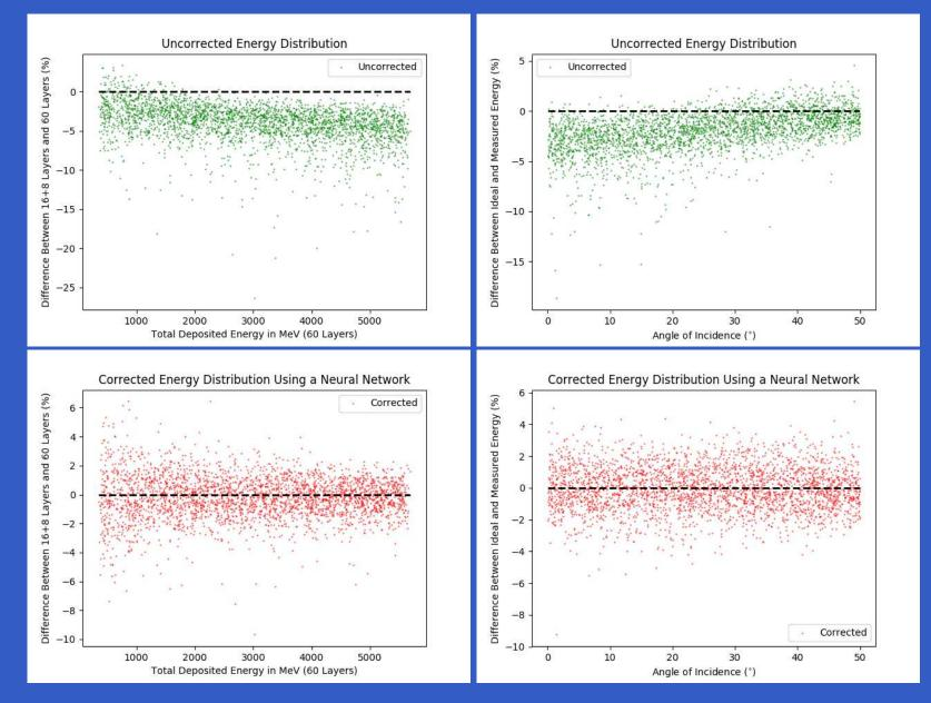
Large leakage at high energy and low  $\theta$  (angle of incidence) can be corrected using a NeuralNetwork prediction of leakage.LCWS19 October 2019 – p.11/18
