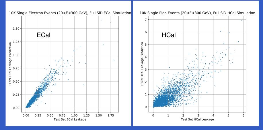
Nominal SiD HCal uses 40 layers of absorbing Steel alternating with sensitive layers. Ideal SiD HCal uses 80 layers, for use in training Neural Network to predict leakage Including intervening ECal layers ( $\approx 1\lambda$ ), unused in right plot, should improve the correlation.
