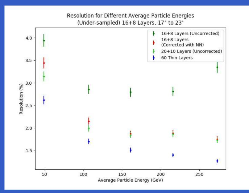
Improvement in resolution similar to simple stack. The reduced SiD ECal performance is comparable to the nominal performance with leakage corrections. LCWS19 October 2019 – p.15/18
