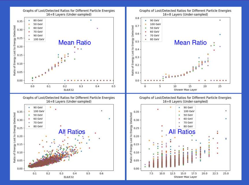
Uniformity of shower profiles yield correlations between energy deposits in layers. EL6 is energy in last 6 layers, E32 is energy in first 32 layers. LCWS19 October 2019 – p.10/18
