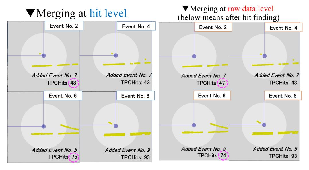
Merging at hit level and raw data level has slightly different track shapes and the number of hits.
