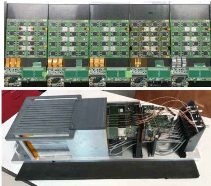
Figure I-5.22. Technological prototype of the SiW ECAL. Top: set of integrated sensor&readout boards; bottom: 10-layers calorimeter prototype used in beam tests at DESY and CERN.
