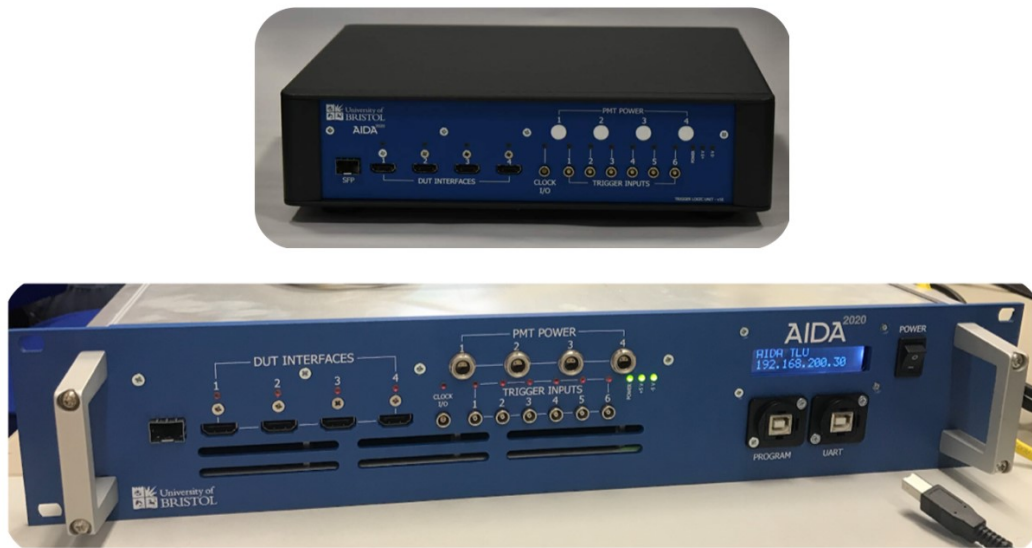
Figure I-6.23. The AIDA-2020 newly developed Trigger Logic Unit. Top: table top enclosure. Bottom: 19-inch rack-mounted enclosure. The two enclosures have identical inner components and provide the same functionalities.
