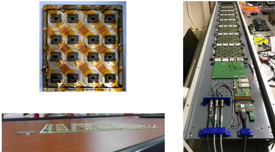
Figure I-5.24. SiW-ECAL developments towards the final detector: thin chip-on-board sensors (left) and long slabs corresponding to ILD dimensions (right).
