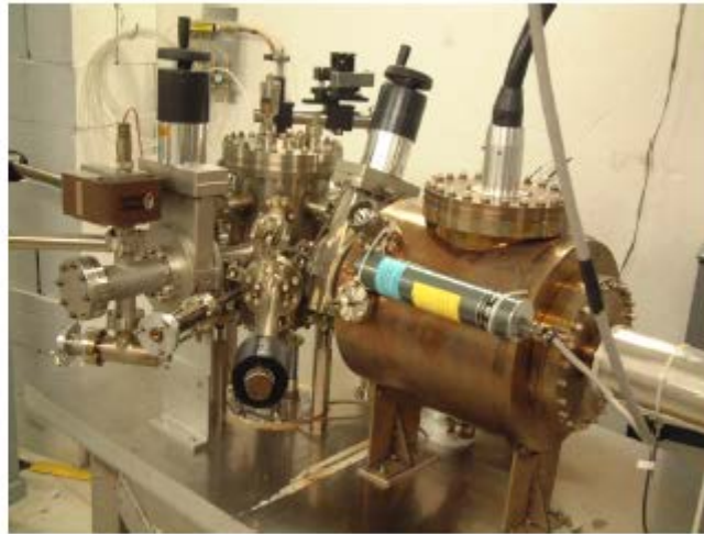
Figure 4.4 The chamber of the 200 kV DC high voltage photogun (a) and its schematic view (b).
