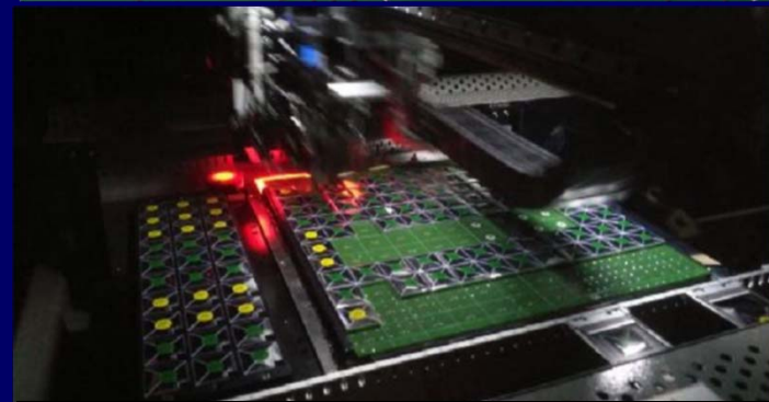
Robot for tiles HCAL construction
