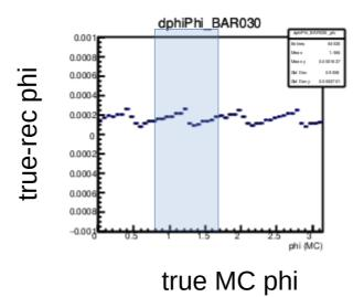
periodic structure due to ECAL structure
