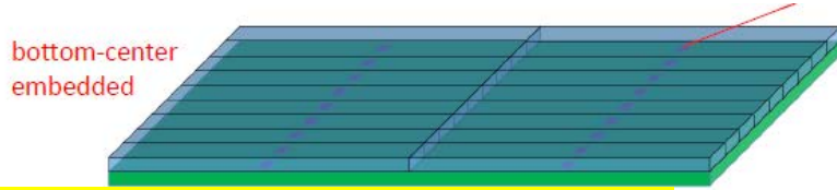
SiPM coupling with scintillator strips
