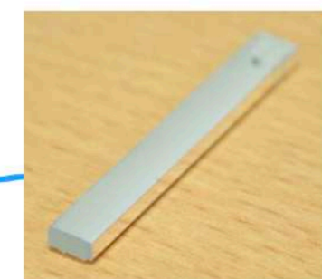
Scintillator (45 x 5 x 2 mm 2 )
