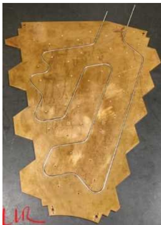
Pipe insertion on a cooling prototype
