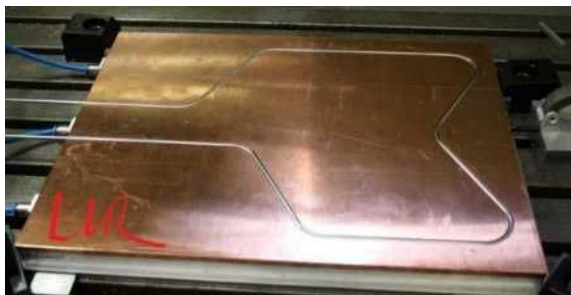
Pipe insertion on a cooling prototype for FEA correlation
