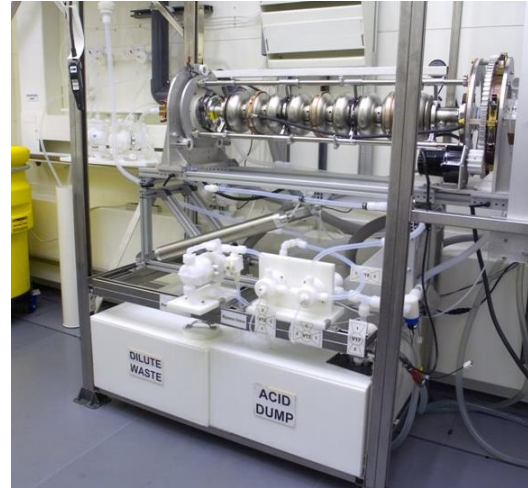
Superconducting cavity processing at the ANL facility jointly funded and staffed by Argonne and Fermilab. Four full time staff (2 ANL, 2 FNAL)
