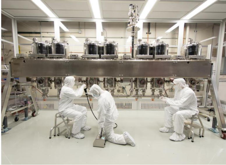
Assembly of ANL-designed ATLAS Intensity Upgrade 72 MHz Quarter-Wave Resonator Cryomodule (2014)
