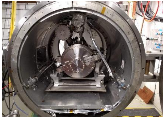
Jacketed HB650 Cavity in STC
