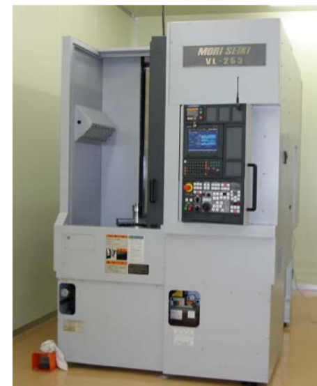
CNC vertical lathe (Moriseiki, Japan)
