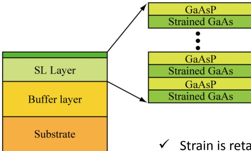
*GaAs-GaAs<sub>x</sub>P<sub>(1-x)</sub> Strained SL*
