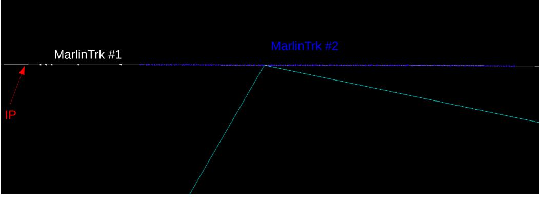
here reco track is broken between si and TPC true decay is in TPC
