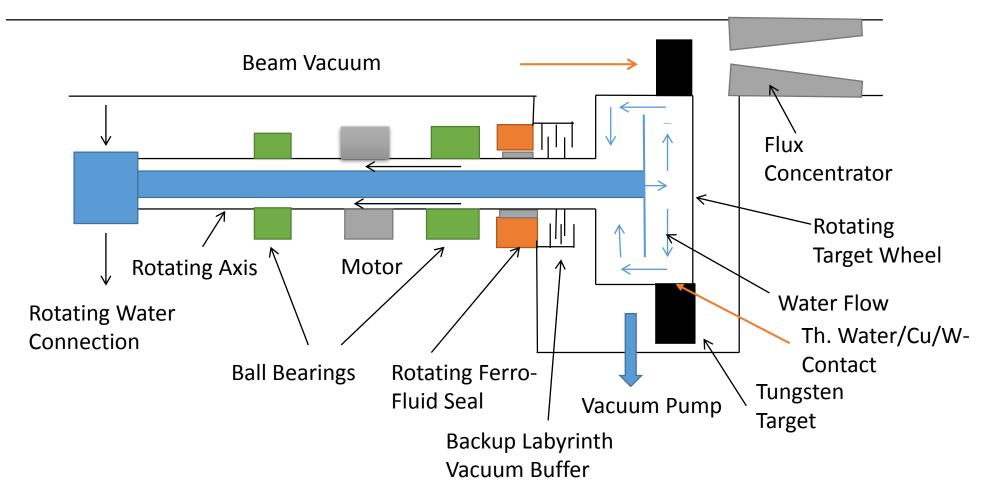
Critical Issue of Rotating Seal: Leak tightnes for UHV. Radiation resistance and radiochemistry of iron powder in oil, and permanent magnets (was tested Omori-san).
