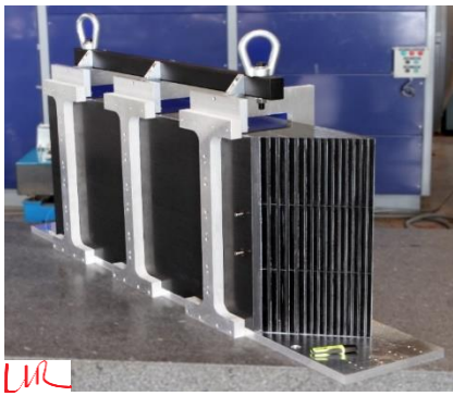
Same concept / EUDET module for barrel (LLR) bag molding & autoclave but different shapes and length of alveoli
