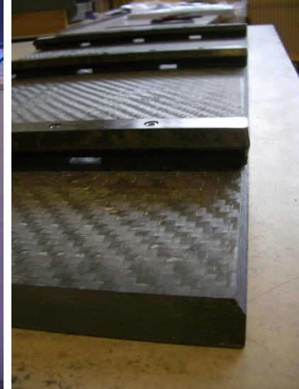
Thick Carbon HR plate Th. 13 mm , with inserts and composite rails done by thermocompression
