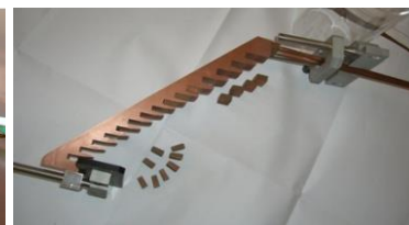
(Left) Design of connection of heat exchangers with one copper drain extremity (Middle) heat exchanger for 15 (x2) connections with Inlet and Outlet pipes on the upper side (Right) localisation of cooling system on one module
