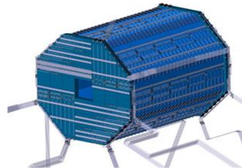
Cooling lines and rails for ECAL End-cap and Barrel
