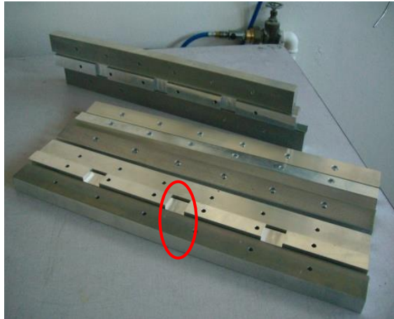
Full Prototype EUDET with opening in rails for the cooling pipes and services' path facing each column
