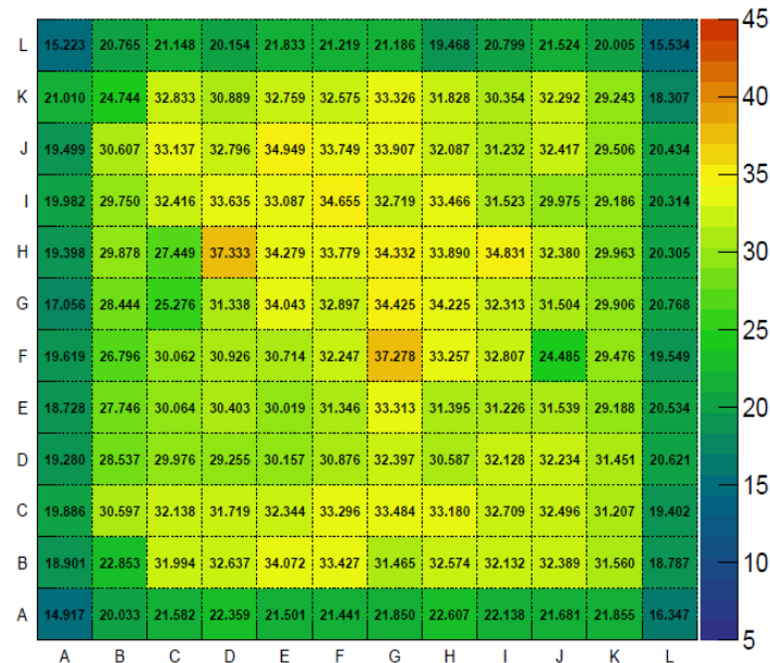
Light yield Map Megatile 6: unpolished surface and dimples, new foil on edge, LY4
