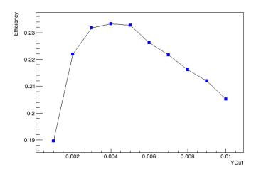
The new  $y_{cut}$ , with the AHCAL simulation, shows a similar shape. But different maximum  $y_{cut} = 0.004$ .
