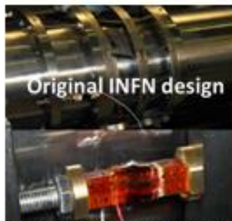
1) Shearing Forces applied to piezostack
