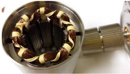
Phytron stepper motor internal windings after irradiation with dose 5 \cdot 10^8 Rad
