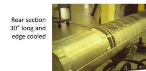
Top view of HX plates. Thinnest plates 3/16" thick
