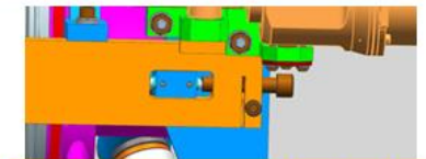
Function of this screw to unload tuner to replace piezo/motor
