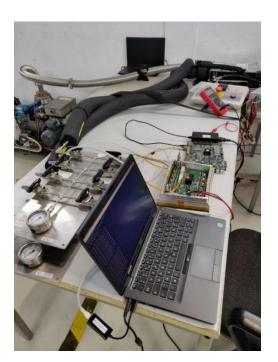
Saclay successful 2-phase CO2 cooling test of a Micromegas module at DESY mid-October with a 3D-printed cooling
