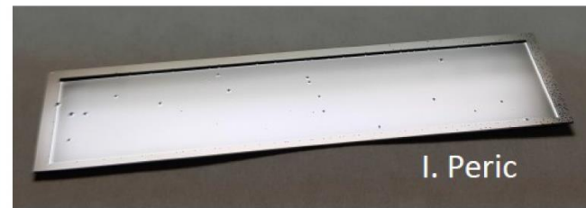
Thinned multi-chip CMOS sensor, I. Peric (KIT) & IZM
