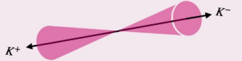
Figure 7 Schematic diagram of s\bar{s} production after its hadronization. Neutral kaons are being ignored for the time being. In reality, these jets will include mixture of pion and proton even in the pure s\bar{s} events.
