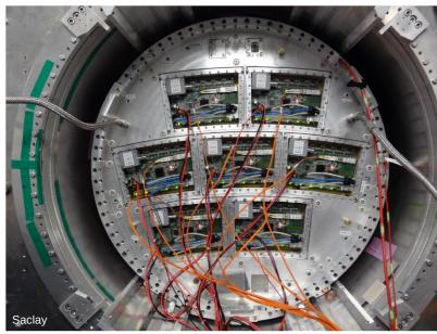
A new HV scheme of the module (ERAM) places grid on ground potential and reduces field distortions between modules by a factor of 10.
