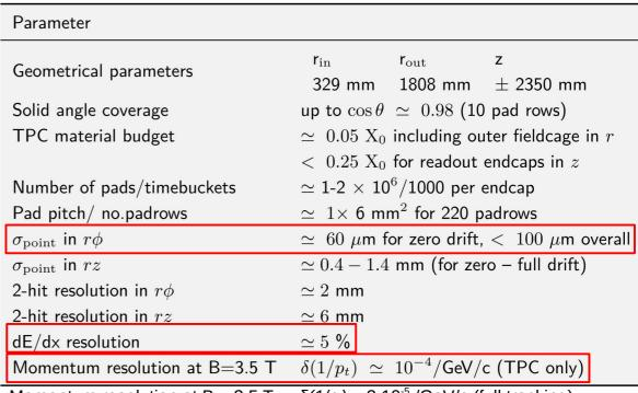
Momentum resolution at B = 3.5 T  $\delta(1/p_i) \approx 2.10^{-5}$  /GeV/c (full tracking) In addition: very high efficiency for particle of more than 500 MeV. These requirements can not be fulfilled by conventional wire-based read out.
