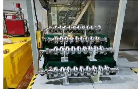
Horizontal test stand, 1.3GHz 9cell cavities, and couplers...
