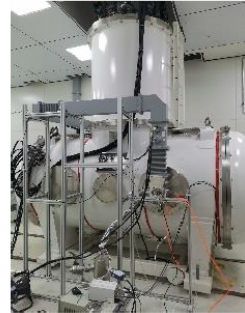
Horizontal test stand, 1.3GHz 9cell cavities, and couplers...
