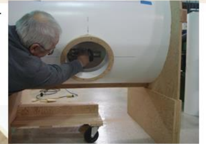
Tuner installed on the CM mock-up at FNAL
