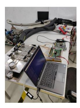
Saclay successful 2-phase CO2 cooling test of a Micromegas module at DESY mid-October with a 3D-printed cooling
